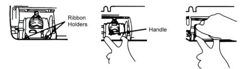
3. Correctly insert a new cartridge between the ribbon guide and the printer head.
